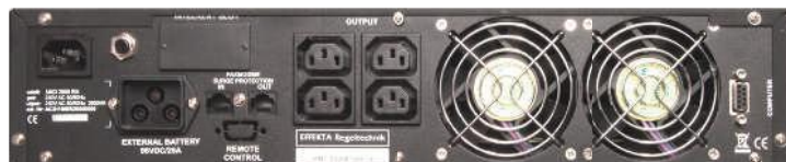
Rear view of MKD 2000 RM (electronics only)
