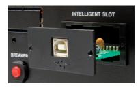
MTD is equiped with RS-232 slot interface, which can be replaced with optional adapters: relay-card, opto-coupler, USB or SNMP.
